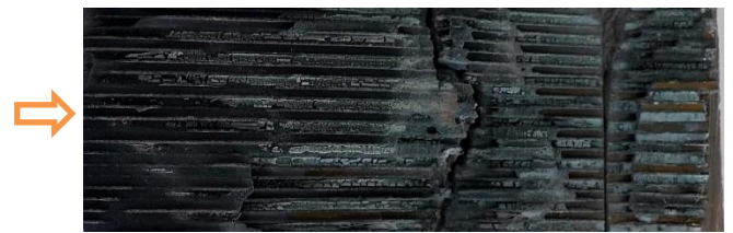
Figure 13. Side of segment 24, slice C to E, showing the substrate melting and the internal of the channels after furnace regeneration.
