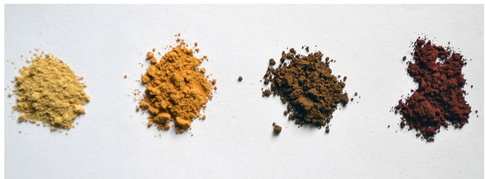
Fig. 1 Commercial ochre pigments (Kremer Pigments). From left to right: light ochre from Cyprus (Kremer code: 17000), burgundy yellow ochre (11573), Cyprus raw umber (40610), and red mine ochre (40351)
