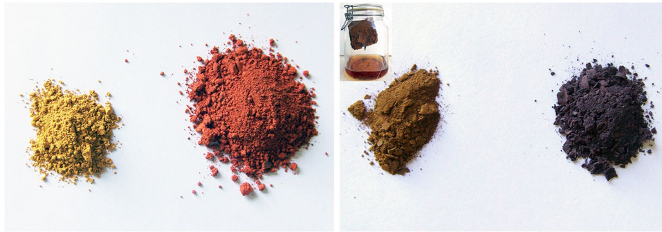
Fig. 4 Left: “French ochre”, Kremer Pigments (product code: 40010), before (left, major components identified by XRD: goethite, quartz, kaolin) and after firing at 920°C (right, XRD: hematite, quartz). Right: artificial iron oxy hydroxide prepared by the vinegar route
