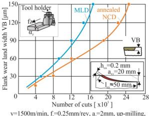
$D_{tool}=100$  mm, dry, t= 5 µm, Workpiece: Aluminum foam
