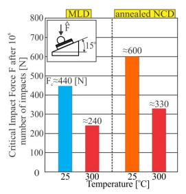
Fig. 4. Determined critical impact force for avoiding coating damage after 10<sup>6</sup> impacts at 25°C and 300°C.
