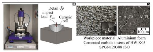
Fig. 1. (a) The employed impact tester for conducting experiments; (b) the workpiece material used in milling experiments.
