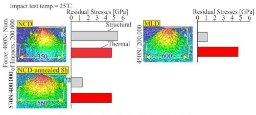
Diamond film: t $\approx$ 5 µm, Rz/Rt=1/1.2 µm, E=1100 GPa Substrate: HW-K05/K20, E=580 GPa, S<sub>y</sub>/S<sub>M</sub>= 3.3/5.8 GPa
