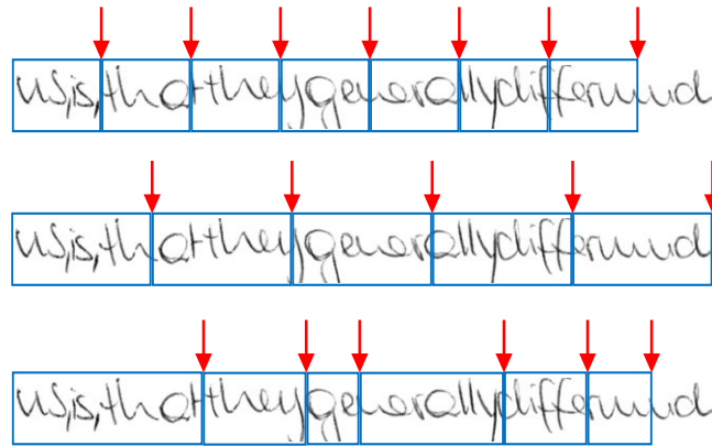
Figure 4-5: Three strategies of cropping a SSOT based on the aspect ratio value are demonstrated. The arrows indicate the position of cropping, and the boxes contain the cropped results, i.e. cropped segments. Top and Middle scheme have fixed value of aspect ratio, which is defined by the user, and so the width of each cropped segment equals to the multiplication of its height with the aspect ratio value. Bottom scheme shows the cropping process when random values of aspect ratio are utilized, and each cropped segment has a different width.
