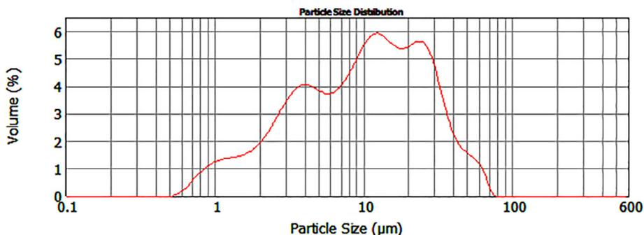
Fig. 1. Particle size distribution of cement I42.5 N.
