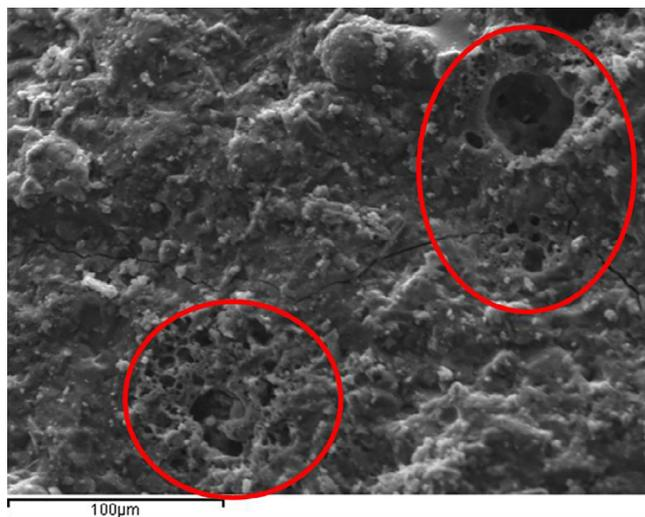
Fig. 7. SEM-micrograph of NC-modified cement paste at 28 days.
