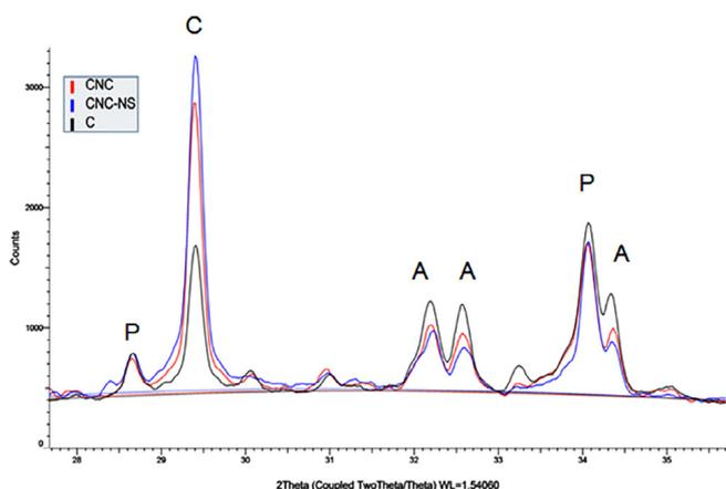
Fig. 5. X-ray diffractograms of nanomodified cement pastes at 28 days.
