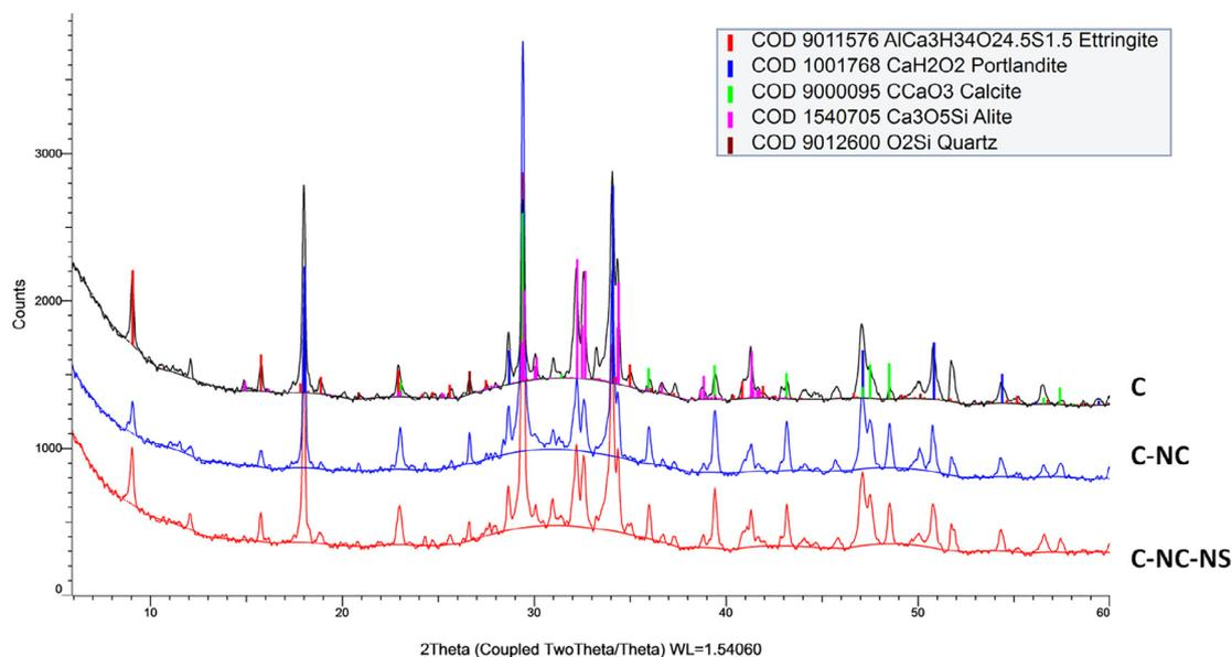
Fig. 4. Mineralogical composition of nanomodified cement pastes at 28 days.
