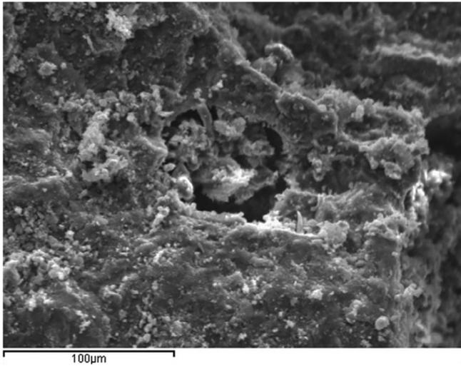
Fig. 8. SEM-micrograph of NC-NS- modified cement paste at 28 days.
