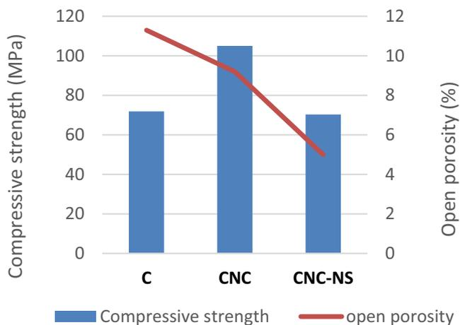
Fig. 3. Compressive strength and open porosity values of reference cement pastes (C) and nanomodified systems with 1.5%wt NC (C-NC) and combination of 1.5%wt NC and 1.5%wt NS (C-NC-NS), at 28 days.
