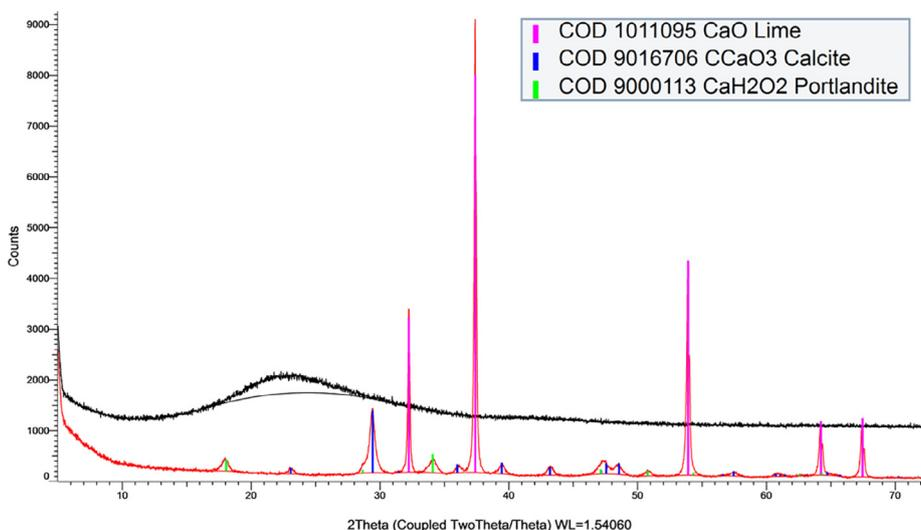
Fig. 2. Diffractograms of NC (red line) and NS particles (black line). (For interpretation of the references to colour in this figure legend, the reader is referred to the web version of this article.)
