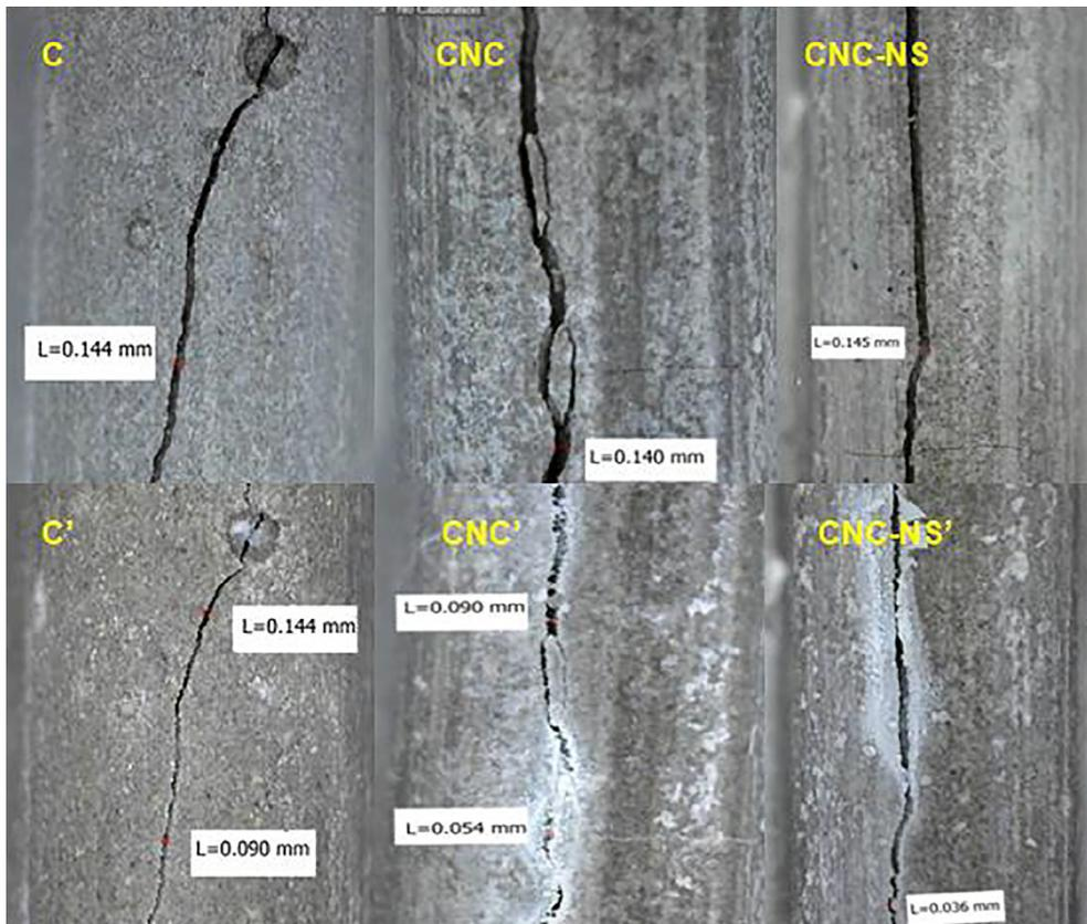
Fig. 9. Microscope pictures of cement pastes after 7 days subjected to water.
