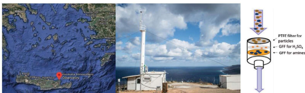
Figure 1. from left to right: The location of Finokalia station on the northeast coast of Crete, view of the station, and sample collector with a triple filter holder used for gas-phase amines sampling.
