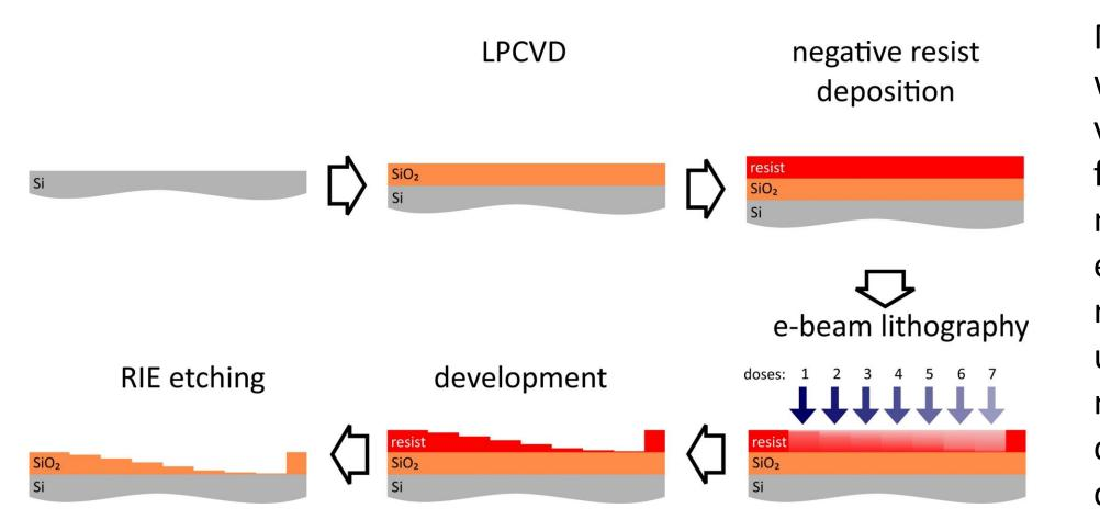
Multilevel resist profiles with defined steps of various heights were fabricated using "tailormade" exposure doses. This exposure dose modulation results in a locally nonuniform etch rate of the resist leading to removal of different resist quantities during the development.
