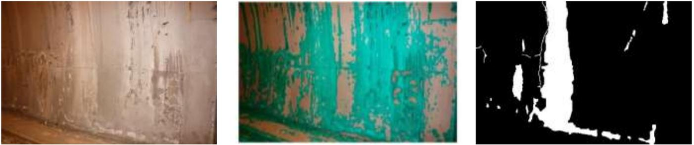
Figure 3.1. (left) Original image from tunnel surface; (center) LDS annotation; (right) Ground truth
