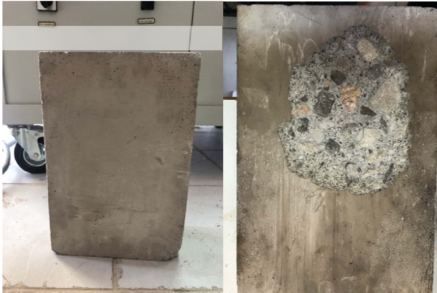
Figure 3 : Concrete C35/45 before and after the fire test
