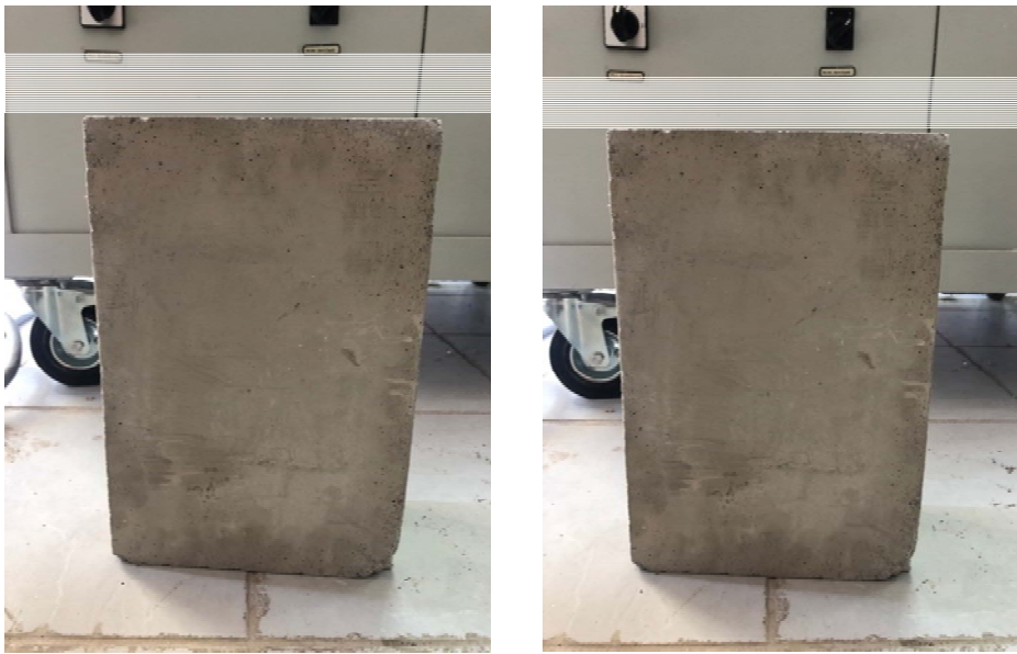
Figure 4: C35/45 before and after the fire test at 400°C
