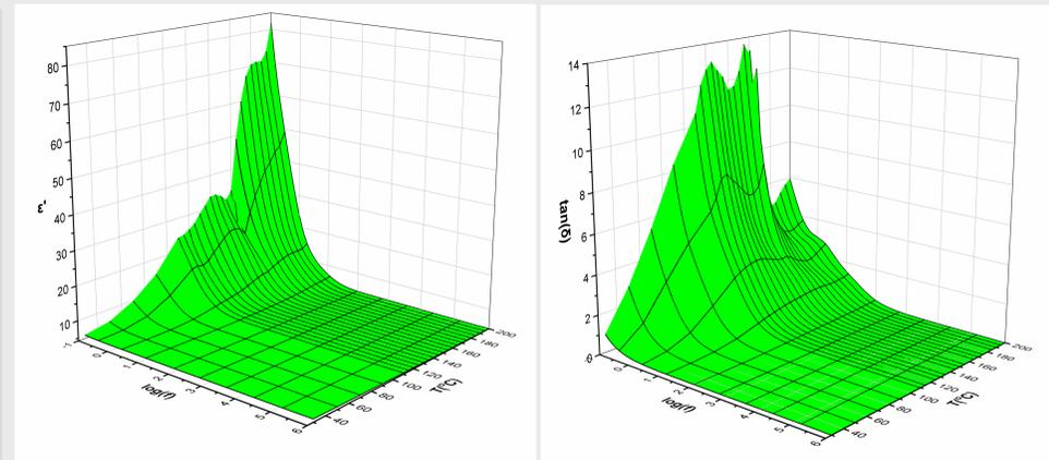
Figure 3. Dielectric spectra of the 1 phr BaTiO<sub>3</sub> nanocomposite as a function of temperature and frequency for the (a) real part of dielectric permittivity and (b) loss tangent.
