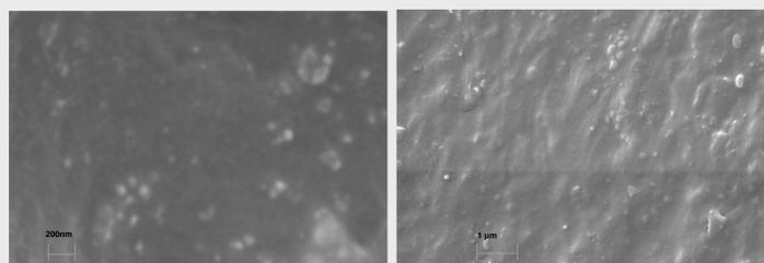
Figure 1. SEM images for the specimens with 1 phr nano BaTiO<sub>3</sub> / PDMS.
