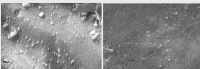
Figure 2. SEM images for the specimens with 1 phr micro BaTiO<sub>3</sub> / PDMS.
