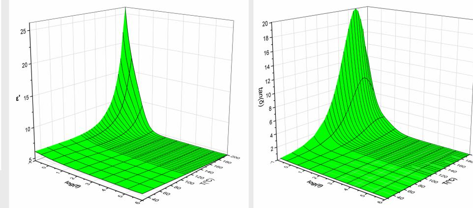
Figure 5. Dielectric spectra of the 1 phr MWCNTs nanocomposite as a function of temperature and frequency for the (a) real part of dielectric permittivity and (b) loss tangent.
