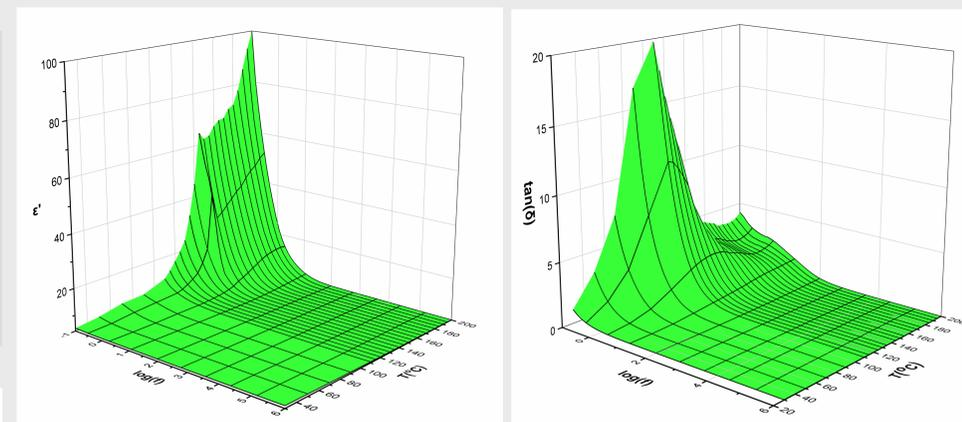
Figure 4. Dielectric spectra of the 1 phr BaTiO<sub>3</sub> microcomposite as a function of temperature and frequency for the (a) real part of dielectric permittivity and (b) loss tangent.
