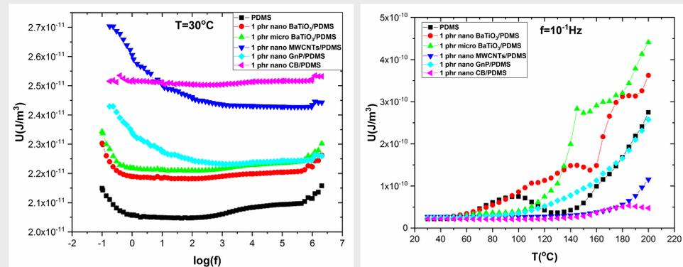
Figure 6. Energy density for all types of fillers a) left as a function of frequency at 30 °C and b) right as a function of temperature at f=0.1 Hz.
