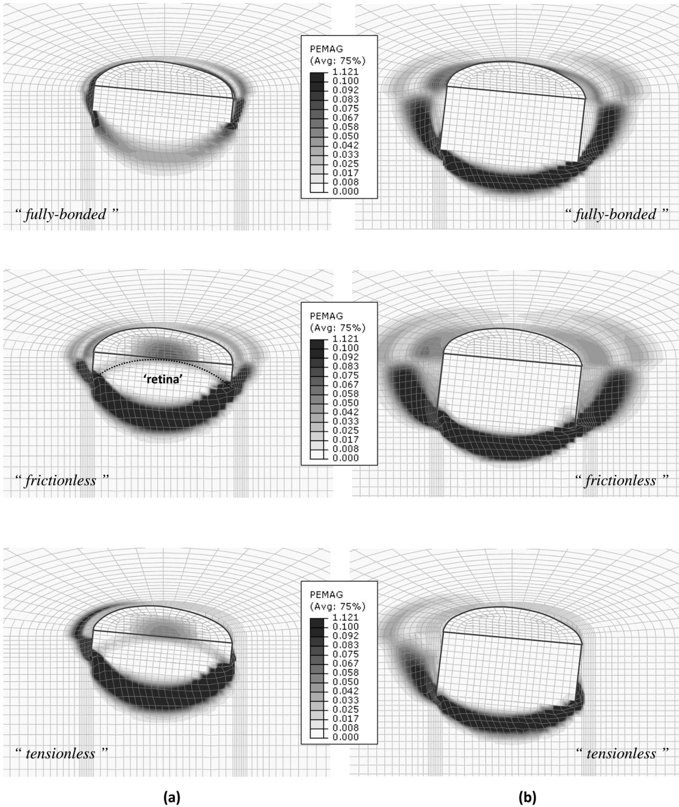
**Figure 12.** Effect of interface conditions on the rotational bearing mechanism of a skirted footing with (a)  $L/D = 0.2$  and (b)  $L/D = 0.5$ .
