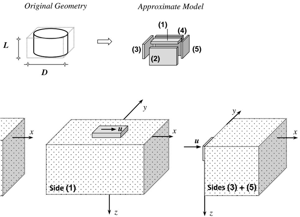
**Figure 10.** Definition of the “Approximate Model” and schematic view of the contribution of each side on the total foundation stiffness : application to horizontal stiffness
