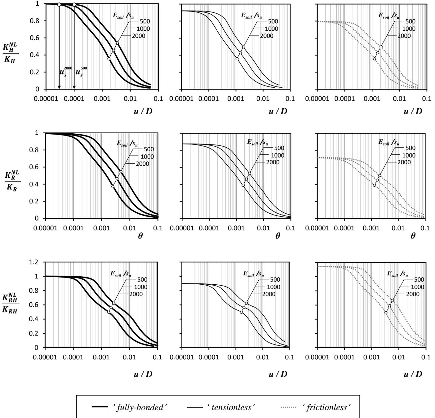
**Figure 14.** Nonlinear stiffnesses of a rigid skirted foundation with embedment ratio  $L/D = 0.2$ : The combined effect of soil rigidity index ( $E_{soil}/s_u$ ) and interface conditions. Results for the ‘tensionless’ interface assumption refer to stability factor  $s_u/\gamma'L = 1.5$ .
