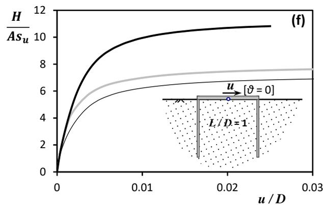
**Figure 8.** The effect of the dimensionless stability parameter  $s_u/\gamma'L$  on : contours of plastic deformation and contours of shear stressing along the caisson skirts for caissons with **(a)** high and **(b)** low stability parameter; on the dimensionless stiffness **(c,d)** and capacity **(e,f)** of shallow and deep caissons.
