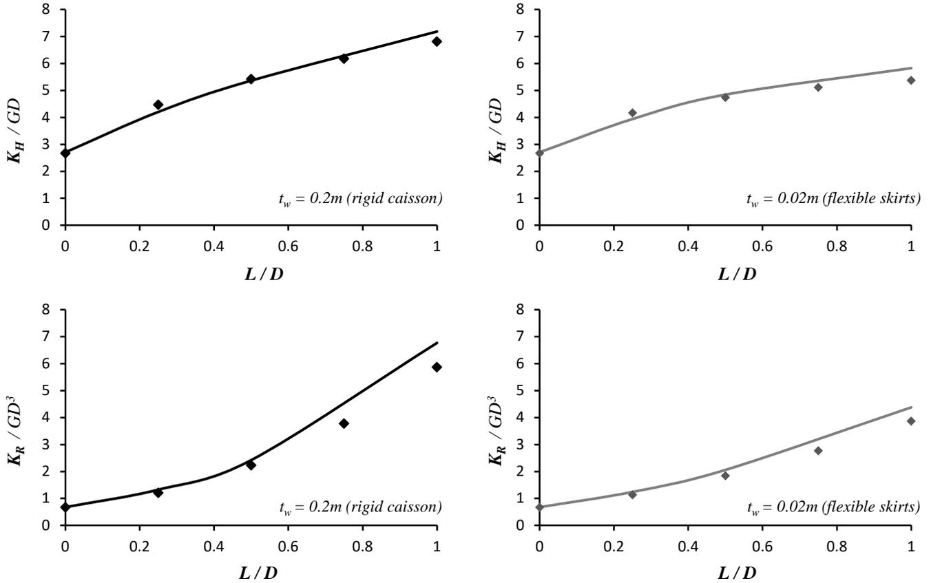
**Figure 4.** Elastic stiffnesses of caisson foundation embedded to elastic half-space: results from this study are compared to the results of Doherty et al (2005).
