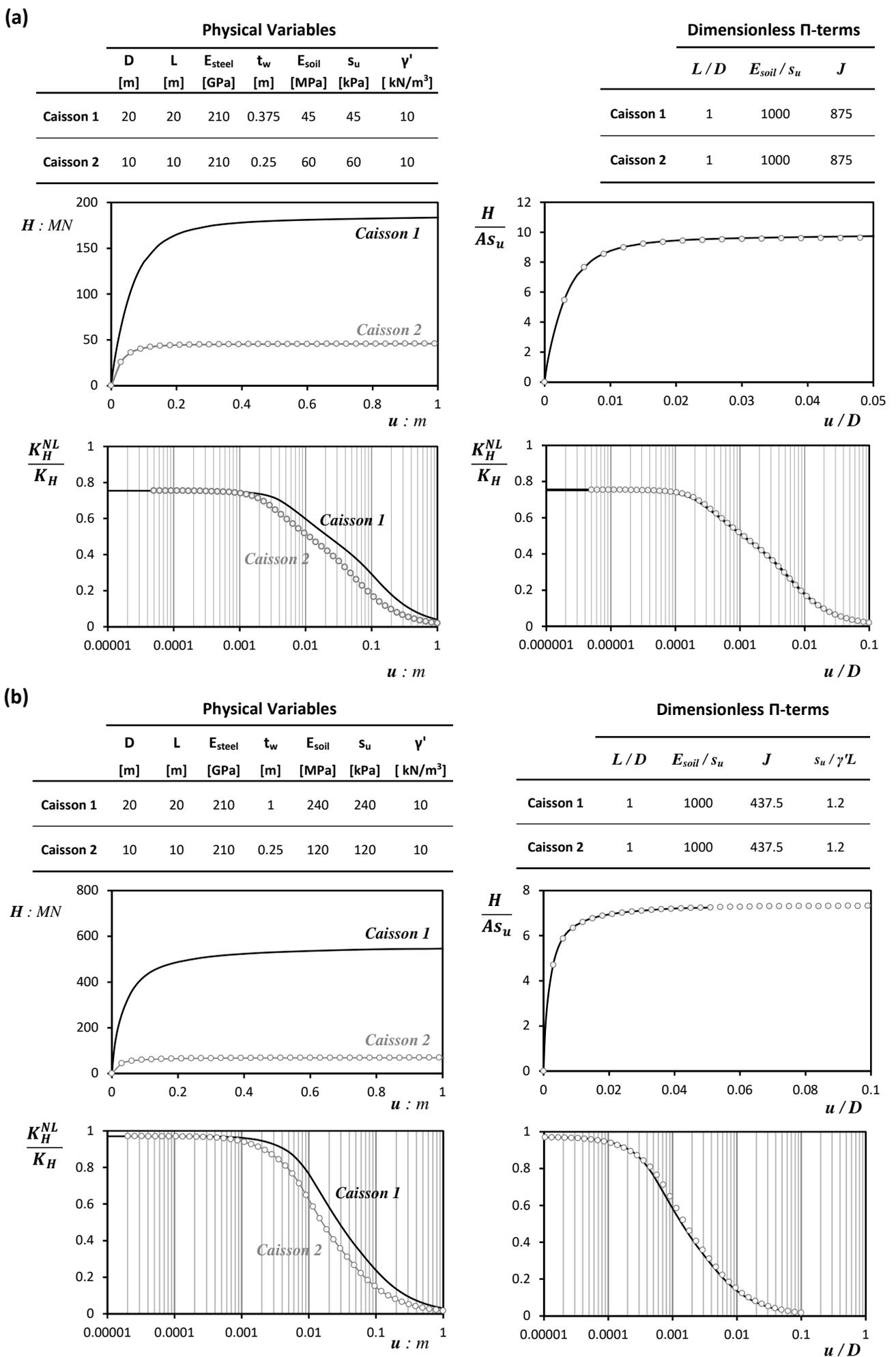
**Figure 7.** Formulation of the dimensionless load-carrying response of a suction caisson in a yielding uniform clay stratum: application to **(a)** ‘frictionless’ and **(b)** tensionless interface conditions
