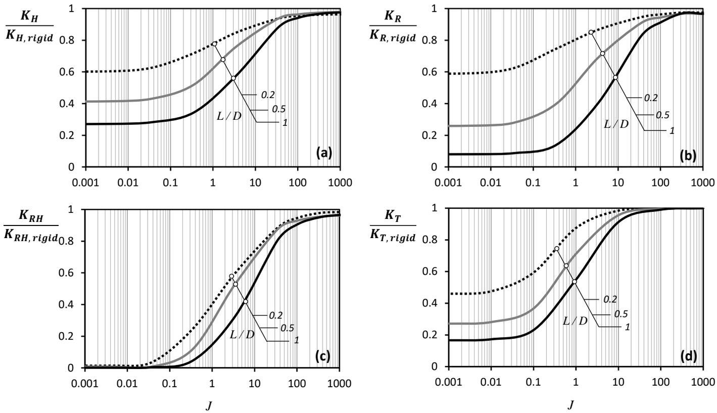
**Figure 6.** Ratios of the elastic stiffness of a skirted foundation “fully-bonded” to soil over the elastic stiffness of the equivalent rigid caisson as a function of embedment ratio  $L/D$  and skirt relative rigidity  $J$ : (a) horizontal; (b) rocking; (c) coupled swaying-rocking; (d) torsional stiffness.
