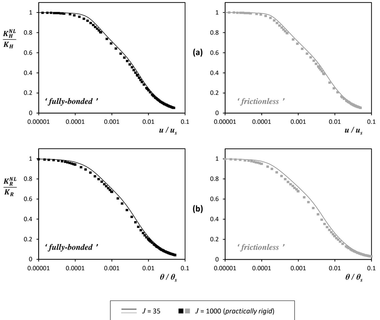
**Figure 16.** Comparison between a practically rigid ( $J = 1000$ ) and a flexible ( $J = 35$ ) caisson with  $L/D = 1$  in terms of nonlinear stiffness  $K^{NL}$ : **(a)** horizontal; **(b)** rotational stiffness, assuming *fully-bonded* (left) and *frictionless* interfaces (right).
