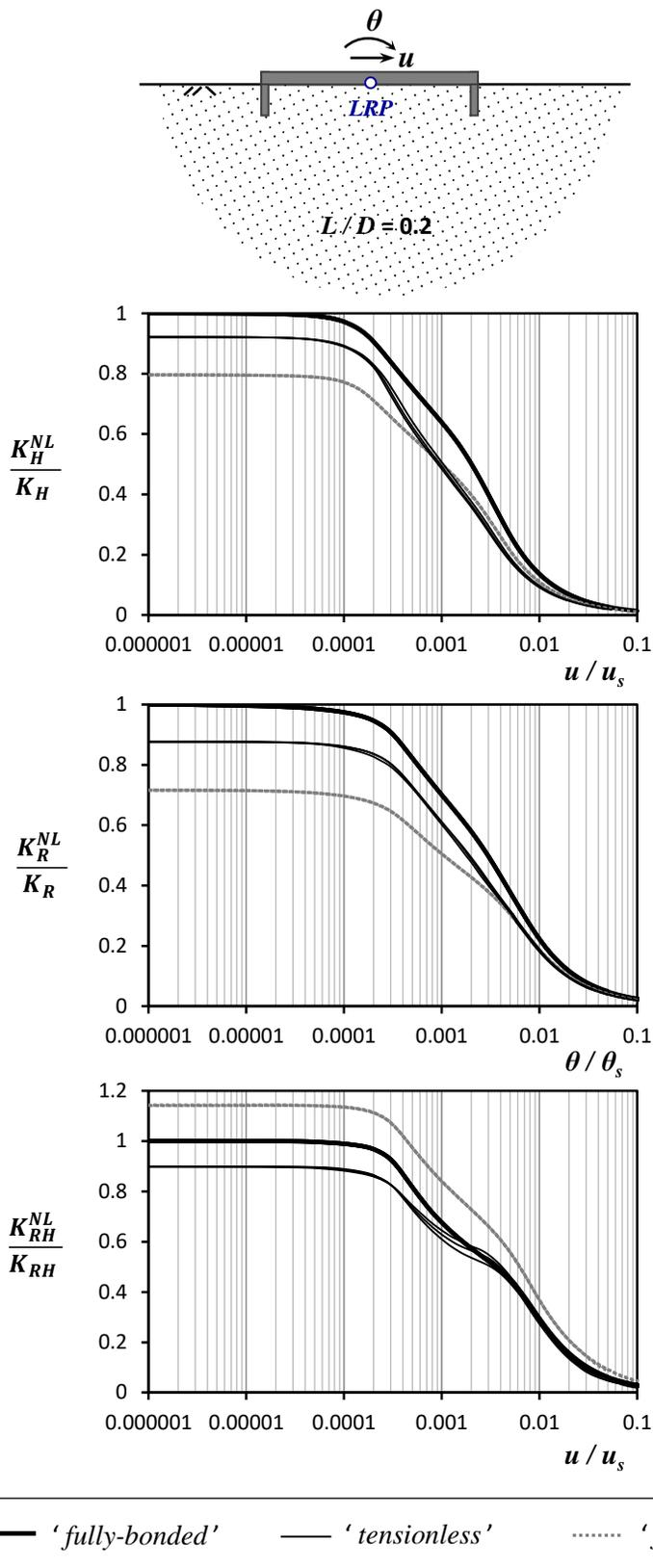
**Figure 15.** Nonlinear stiffnesses of a rigid skirted foundation with embedment ratio  $L/D = 0.2$  expressed in terms of the dimensional quantity  $u/u_s$  or  $\theta/\theta_s$ .
