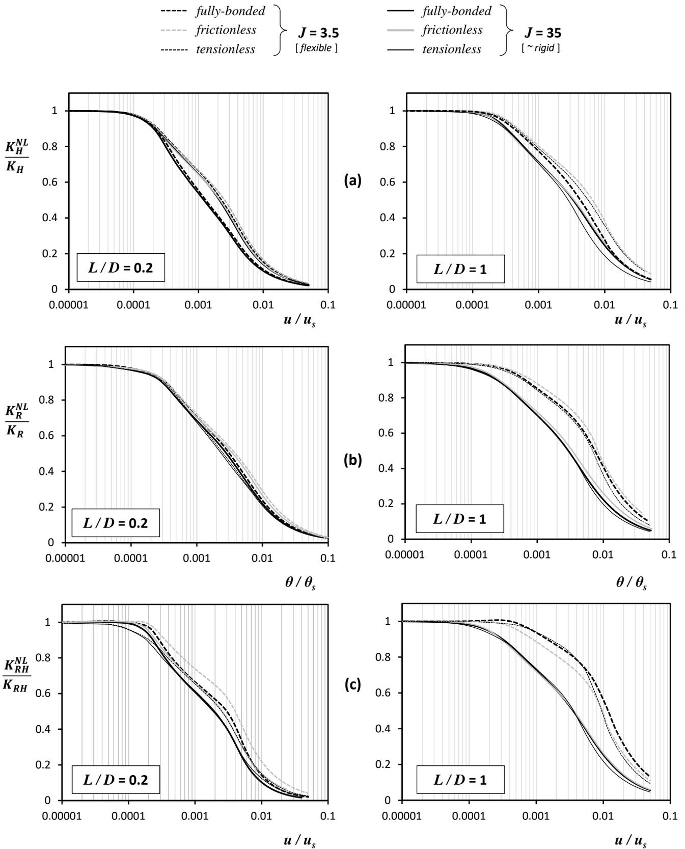
**Figure 17.** Effect of skirt relative rigidity  $J$  on the nonlinear stiffness  $K^{NL}$  of a shallow ( $L/D = 0.2$ ) and a deep ( $L/D = 1$ ) caisson : **(a)** horizontal ; **(b)** rotational ; **(c)** coupled swaying-rocking stiffnesses. The tensionless curves (thin black line) have been derived assuming for the shallow caisson  $s_u/\gamma'L = 1.5$  and for the deeper caisson  $s_u/\gamma'L = 0.3$ .
