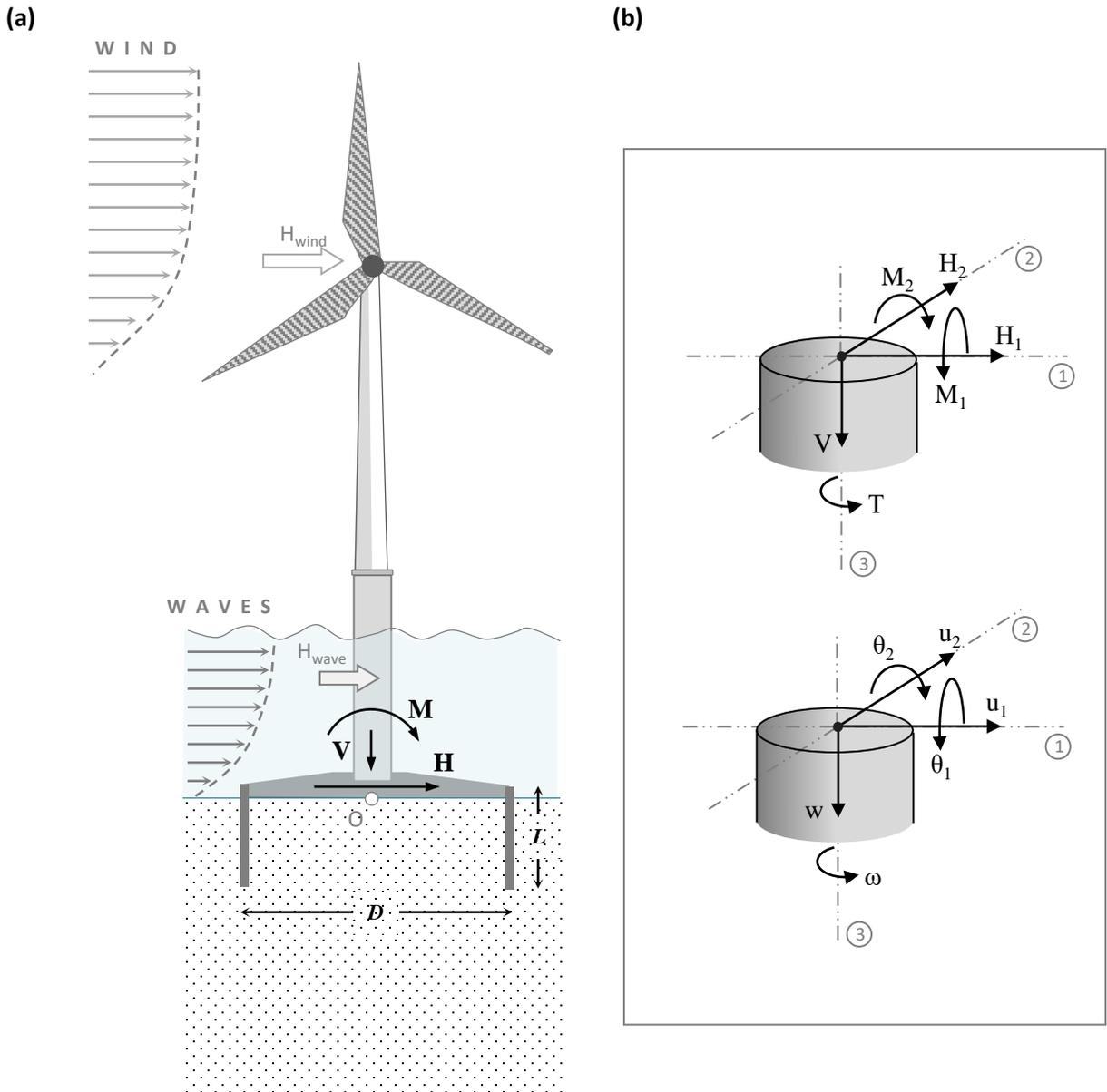
**Figure 1. (a)** A conceptual sketch of the problem under study: an offshore wind-turbine is founded on a suction caisson transmitting V-H-M loading at the top of the foundation; **(b)** nomenclature of generalized loads and corresponding caisson displacements.
