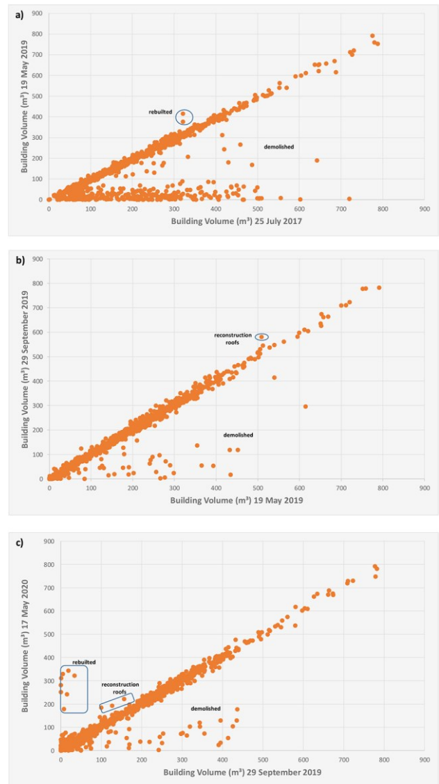
Figure 14. Buildings volume charts which clearly shows the demolition and rebuilt process between the three (3) flight campaigns with UAS, that took place in Vrissa between 2017 and 2020.
