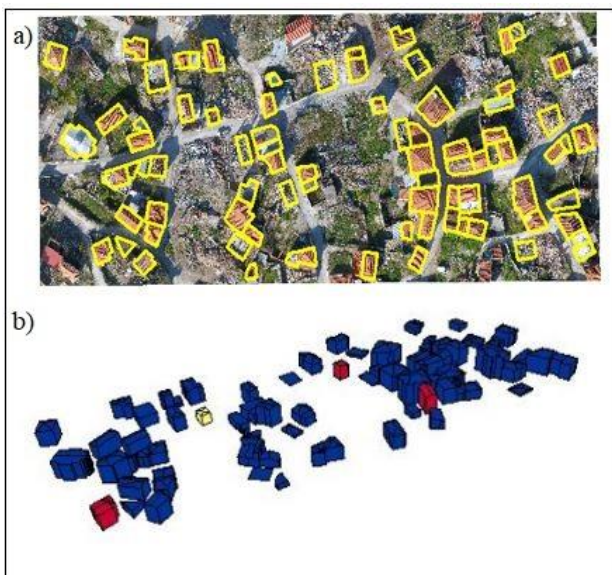
Figure 5. a) Footprints of 80 buildings used for the 3D reconstruction of the two scenarios and b) LOD2 buildings generated by BuildingReconstruction software
