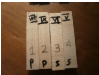
Figure 3. Wood specimens with parallel (P1, P2) and perpendicular (S3, S4) fibers in relation to the longitudinal axis.
